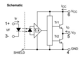
$0.1~\mu F$  bypass capacitor must be connected between pins 6 and 4. (Note 4)
